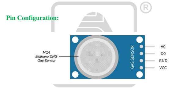
**VCC Pin:** This pin provides voltage to the module and the typical operating voltage is +5V.
