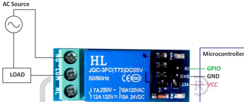
The mains wiring is screwed to the terminal block, and the microcontroller can be connected using jumper cables.
