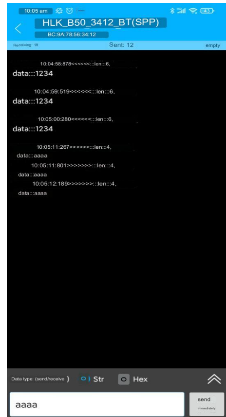
Figure 6 Serial port and APP pass-through data testing
