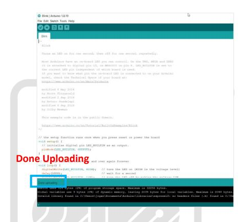
As a result, LED on the ADIY UNO board blinks with specified delay.
