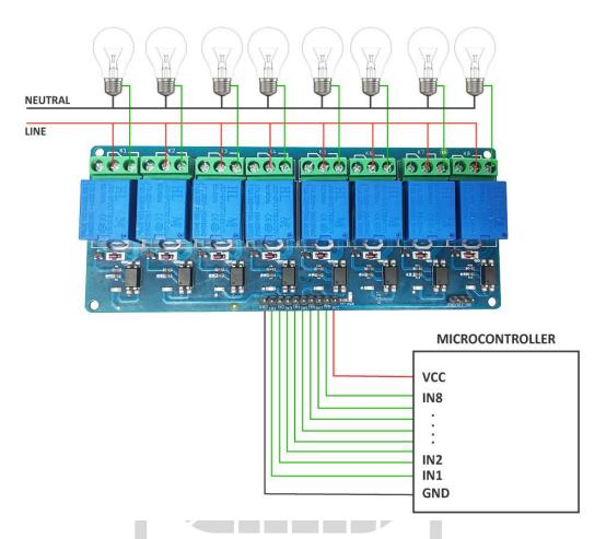
In this diagram, eight separate loads (represented by lightbulbs) have been connected to the NO terminals of the relay. The live wire has been connected to the common terminal of each relay. When the relays are activated, the load is connected to the live wire and is powered. This setup can be reversed by connecting the load to the NC terminal, which will keep it powered on till the relay is activated.
